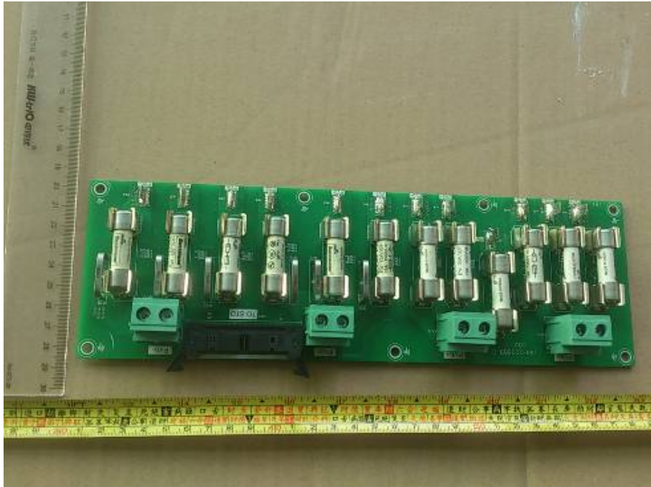
Front view of the fuse board
